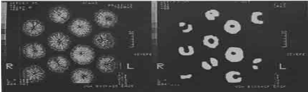
Fig.2 X-ray line scans of Red Delicious apples. Raw images are on the left. Computer enhanced zones of water core are depicted on the right (Shahin and Tollner, 1997)
